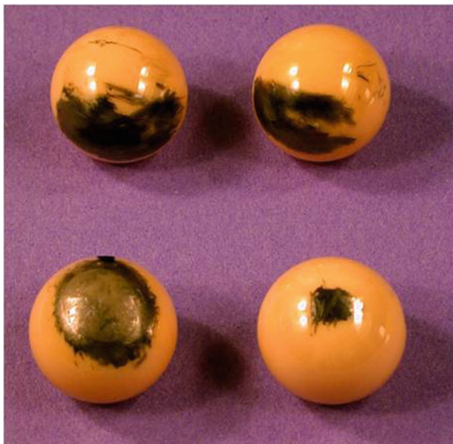
Fig. 15.13 Examples of retrieved ceramic femoral heads that have worn-through the polyethylene acetabular components. There is a transfer layer of titanium from the titanium backing of the acetabular components. Retrieved specimens courtesy of the Anderson Orthopaedic Research Institute
