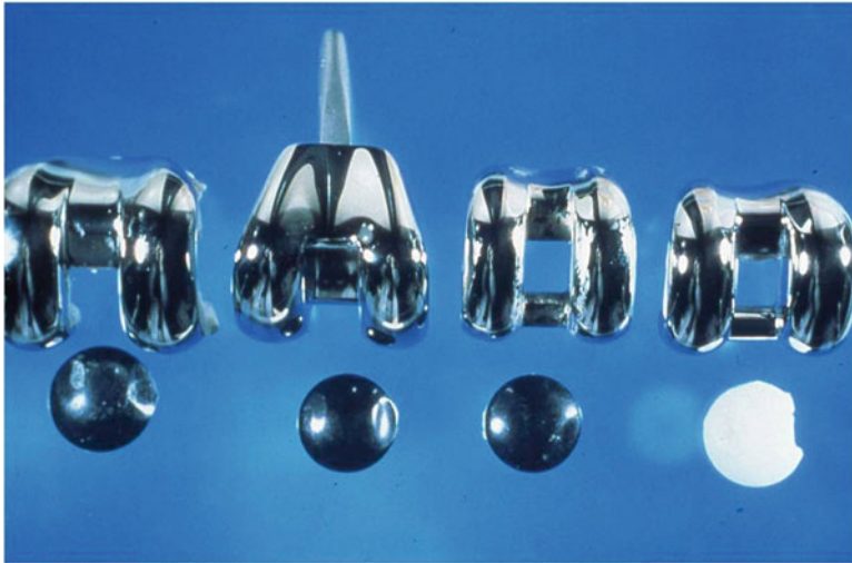
Fig. 15.11 Plastic deformation and failure of thin all-polyethylene patellar buttons against the trochlear groves of the femoral components
