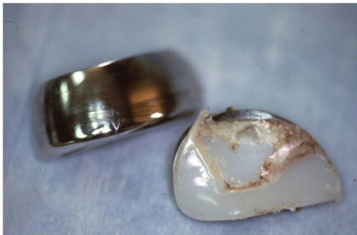
Fig. 15.3 Edge loading of polyethylene with failure to tibial tray and consequent burnishing of femoral component related to malalignment of unicompartmental knee replacement
